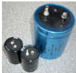
Fig 4: The single large capacitor and the two smaller ones that replaced it.
