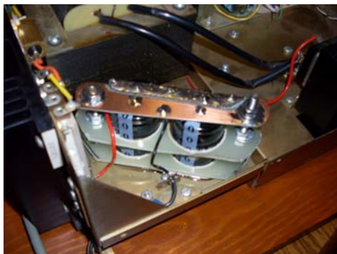
Fig 5: Wes's answer of how to overcome the strain of the original large wires.
