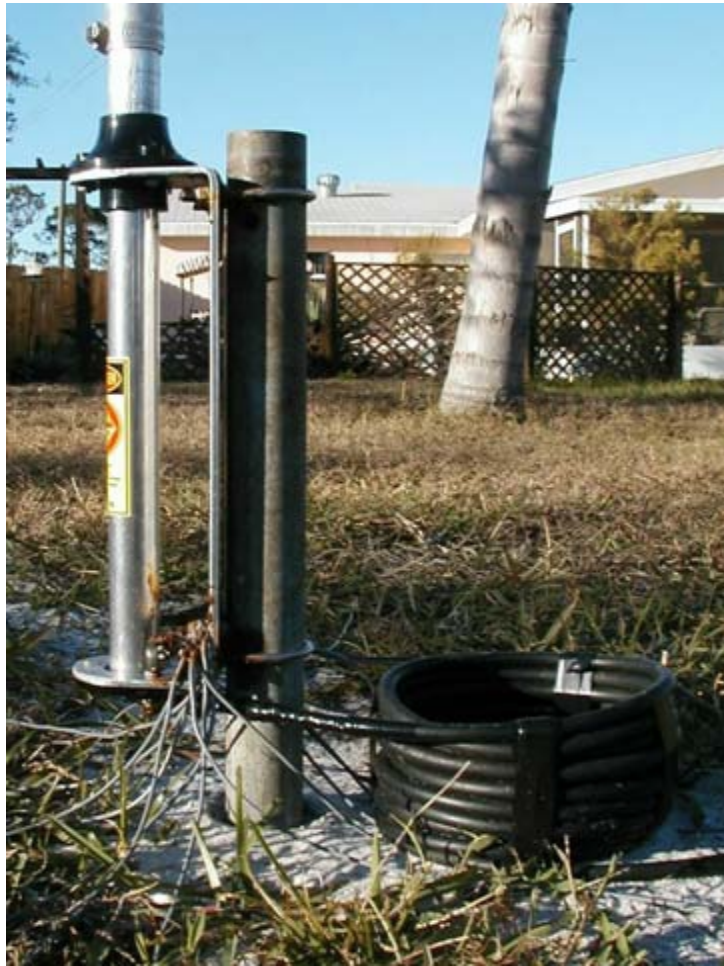
The base of the 5BTV showing the ground post, mounting bracket and decoupling coil.
