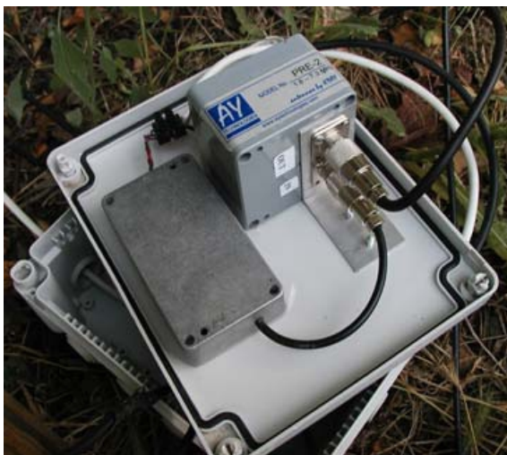
Internal view of the switching unit.
